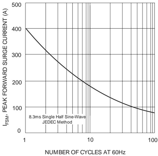
Fig. 3 Maximum Non-Repetitive Peak Forward Surge Current
