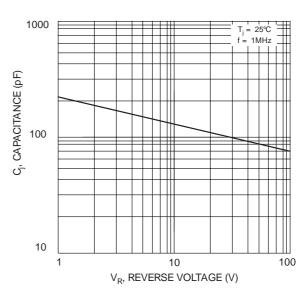
Fig. 4 Typical Junction Capacitance
