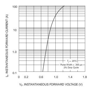
Fig. 1 Forward Current Derating Curve
